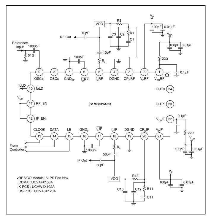
**NOTE:** The role of Rin: Rin makes a large portion of VCO output power go to the load rather than the PLL. The value of Rin depends on the VCO power level.
